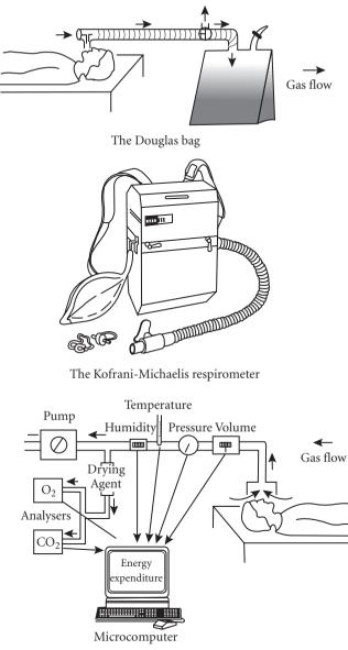
A ventilated hood indirect calorimeter
